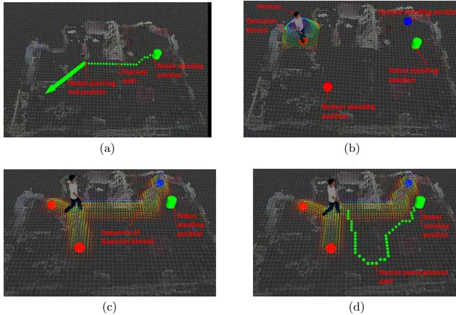
**Fig. 3.** A graphical outline of the steps of the proposed method; a) the robot planning without human presence, b) the model personal area of the human using a Gaussian kernel, c) the sequences of the Gaussian kernels from the human current position to the standing positions and d) a human aware planned path
