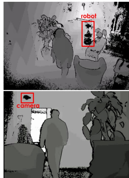
Figure 4. RGB-D camera viewpoint: Top – wall-mounted fixed camera, bottom - robot-mounted camera
